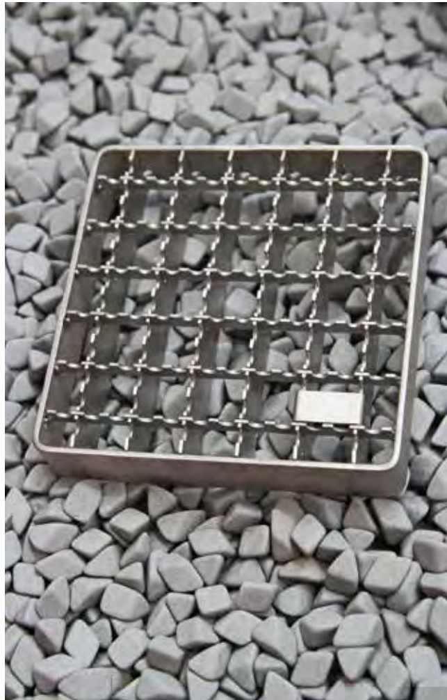
Figure 3. A stainless steel mesh grating during the vibro-abrasive process using ceramic mouldings material.
