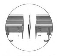
Place the flanges of the channels close together. To avoid mechanical damage, please turn the channels upside down.
