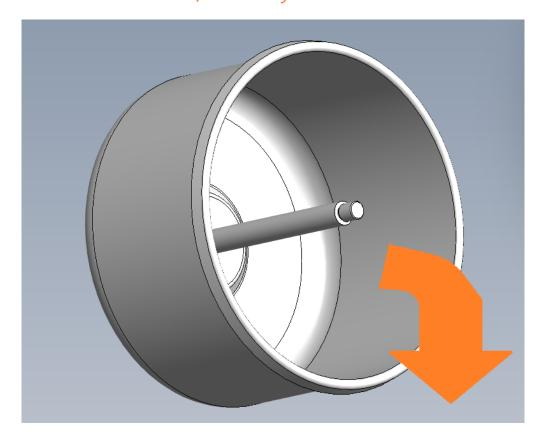
After the washing, lubricate the thread on the stem (copper grease) and the gasket (slip paste for sanitary connections) and screw the elements together again.
