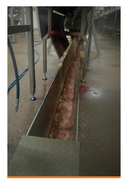
Together with some other tailor-made steel constructions, such as railings and holding tanks. Products were manufactured in stainless steel AISI 304, fully pickled in acid bath for an optimal resistance against corrosion.
