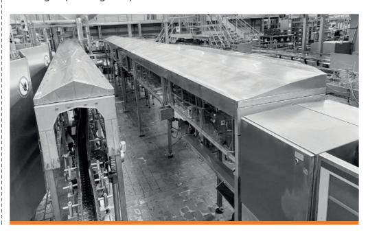
$\cdot$  All elements were tightly fitted to meet the needs of the hygienic work environment. No screws, sharp element etc.
